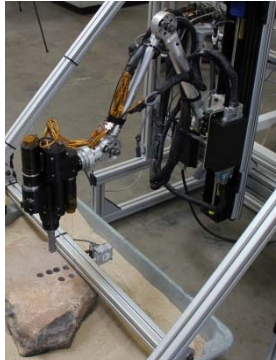
Figure 1. Rotary-Percussive coring drill undergoing testing in 120 MPa basalt. The drill can reach 5cm depth, break-of the core and capture it in 10 minutes
